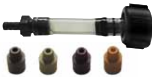
57-11-1 Tip kit for lean dilution ratios 750:1, 1000:1, 1500:1, 2000:1 Includes 4 metering tips, 8 ft. 1/4 inch vinyl hose and 1/4 inch x 3/8 inch barb adapter
